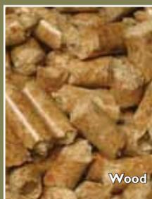
Wood pellets are made of wood by-products (such as sawdust, wood chips, and other wood waste products) of varying qualities. These by-products are run through a pelletizing machine that produces pellets measuring approximately 1/4" diameter by 3/4" long. Pellets can vary in cost, depending on the quality and ash content. They are packaged in 40-lbs. bags for easy handling.
